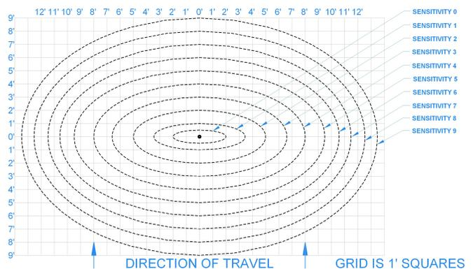
**Response Time:** Output activation within 55 milliseconds of the vehicle entering the detection zone. Output deactivation within 135 milliseconds of the vehicle leaving the detection zone.
