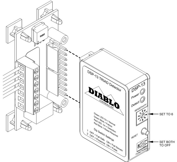
**Step 6** Cycle the gate several times to verify that the gate is not detected. If it is not detected, the sensor can be moved closer to the gate if needed. If detected, move the sensor further away. If it cannot be moved further, turn down the sensitivity and press RESET and retest.
