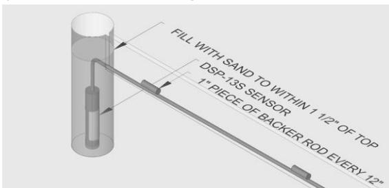
**Step 11** Run the lead-in cable from the exit point in the driving surface to the operator. Installing a conduit will provide an additional layer of protection.
