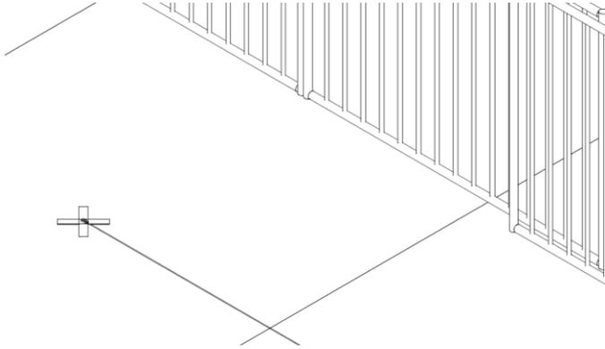
**Step 9** Make a single 1/4" saw cut, a minimum of 2" deep, from the edge of the driving surface to the marked sensor location. Then core drill a 1" to 2" hole, 6" deep.
