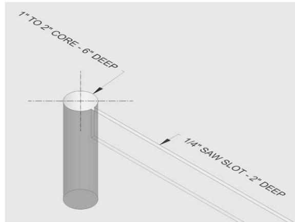
**Step 10** Install the DSP-13S sensor at the bottom of the hole as shown. Fill the sensor hole with sand to within 1 1/2" of the surface. Install a 1" piece of backer rod every 12" to hold the lead-in cable at the bottom of the saw slot. Fill the hole and the saw slot with an appropriate sealant for the driving surface.
