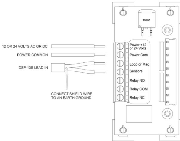
**Step 5** Install the DSP-13M on to the RK1-R. Set the sensitivity to 6 and both DIP switches to OFF. Then press the RESET button.
