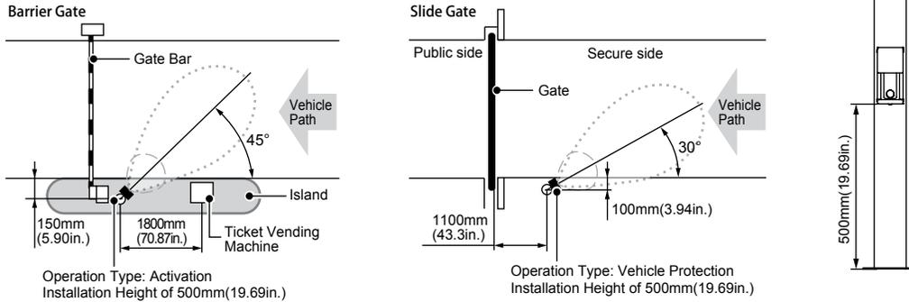
3. If Vehicle protection mode, find the installation location by referring the following chart. Always recommended to install 700mm(70.87") far from barrier or slide gate. Installation height has to be 500mm(19.69") from the ground.
