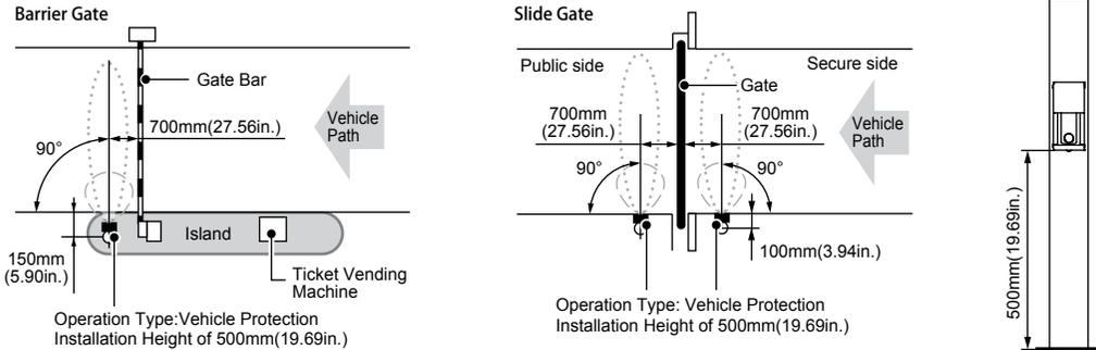
4. Install the sensor, wire it and apply power.
